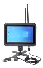
b. Power adapter cable (8Pin to 4 loose wires) directly connect to vehicles power, this requests vehicles to provide stable power within 19V
